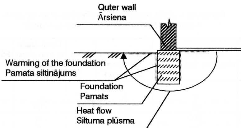
*Fig. 1a. Scheme of the house foundation.
