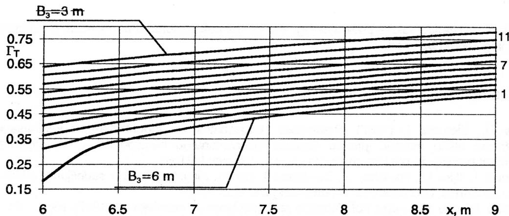
Fig. 8. Dependence of the geometrical coefficient of thermal resistance  $\Gamma_T$  on the width of heat insulation  $x$  horizontally outside a building in combination with heat insulation under the floor.  $x$  - co-ordinate of the point  $B_4$  in Fig. 1. Co-ordinate of the point  $A_5$  is 6 m. Curves 1, 2, ..., 11 - accordingly correspond to additional heat insulation inside a house (alteration of the co-ordinate of the point  $B_3$  is from 6 to 3 m with a step of 0.30 m).
