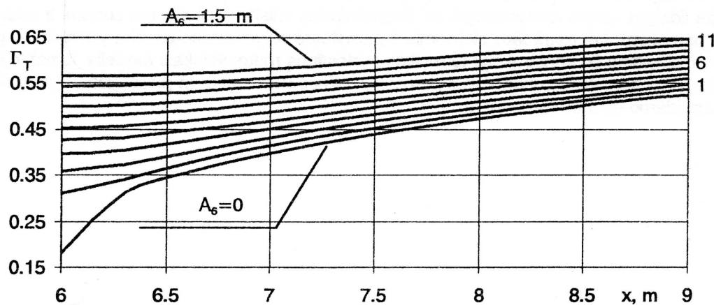
Fig. 9. Dependence of the geometrical coefficient of thermal resistance  $\Gamma_T$  on the width of heat insulation  $x$  horizontally outside a building in combination with vertical insulation of the foundation.  $x$  - co-ordinate of the point  $B_4$  in Fig. 1. Co-ordinate of the point  $A_5$  is 6 m. Curves 1, 2, ..., 11 - correspond accordingly to additional heat insulation of the foundation in the ground at the depth of 0-1.5 m with a step of 0.15 m.
