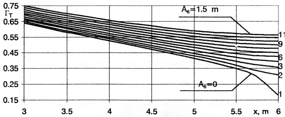
Fig. 7. Dependence of the geometrical coefficient of thermal resistance  $\Gamma_T$  on the width of heat insulation  $x$  horizontally inside a building in combination with vertical insulation of the foundation.  $x$  - co-ordinate of the point  $B_3$  in Fig. 1. Co-ordinate of the point  $A_5$  is 6 m. Curves 1, 2, ..., 11 - accordingly correspond to additional heat insulation in the ground at the depth of 0-1.5 m with a step of 0.15 m.
