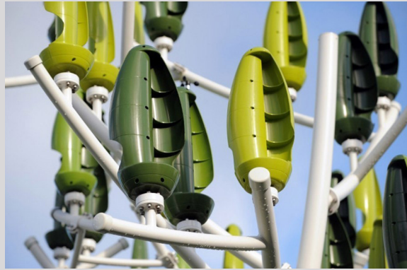
Figure 29, 30. Wind trees with integrated mini wind turbines in France (Meet the wind..., 2016; The wind tree..., 2016)
