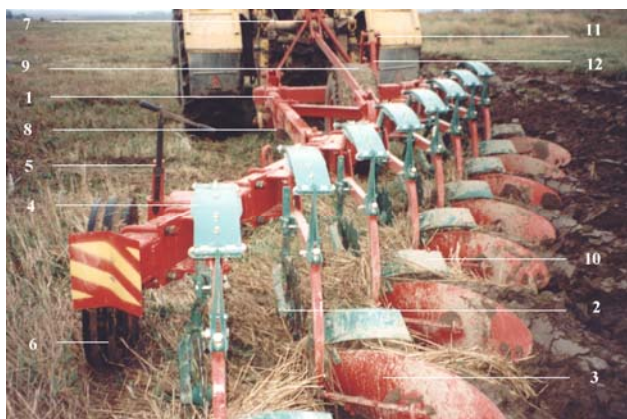
19.att. Arklis AGK–8–40 ar pusskrūves tipa korpusiem Fig. 19. Plough AGK–8–40 with semi-helicoidal bodies
