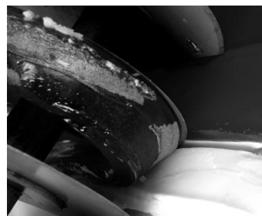
Figure 9. Mixed destruction of adhesive compound in forming combined candy bodies by smearing and cutting methods
