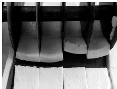
Figure 8. Adhesion failure in forming combined bodies by smearing and cutting methods
