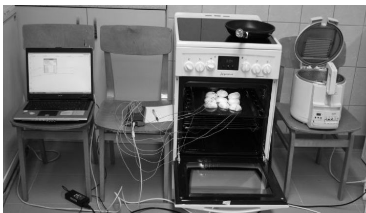
Figure 1. Time/temperature control with TC-08 Thermocouple Data Logger equipment
