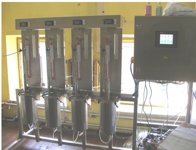
Fig. 1. Part of laboratory equipment B4 for biogas yield investigation
