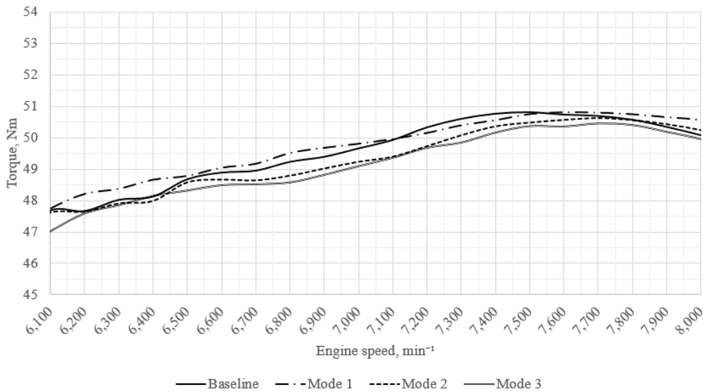
Figure 3. Torque comparison at medium engine speeds.
