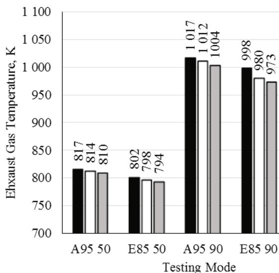
Figure 1. Temperature of engine-out exhaust gases: ignition timing: ■ 31.5...31, □ 34...33, ▒ 36...37.
