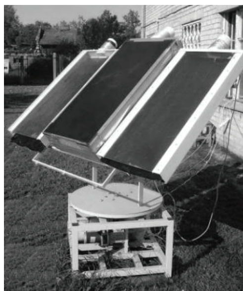
Figure 2. The collector tracking the Sun comparative research in the experiment.
