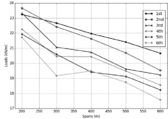
Figure 14. Calculated loads for highway's A3 Lane1
