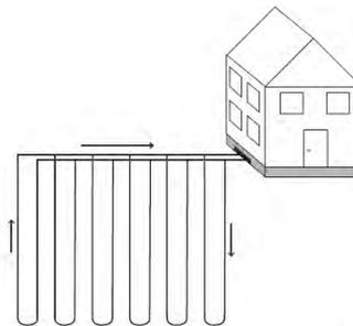
**Figure 5.** Vertical closed loop heat exchange system for geothermal heat pump (Self, 2013)
