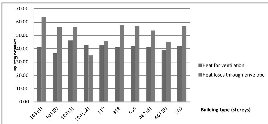
Figure 2. Necessary annual heating energy for optimal ventilation volume and heat losses through building envelope
