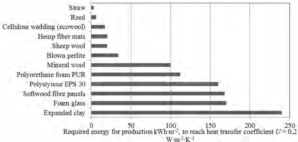
**Figure 4.** Required energy for material production, when heat transfer coefficient  $U = 0,2$  W·m<sup>-2</sup>·K<sup>-1</sup> (Vom..., 2014)
