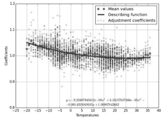
Figure 7. Adjustment coefficients and describing function. A1 data
