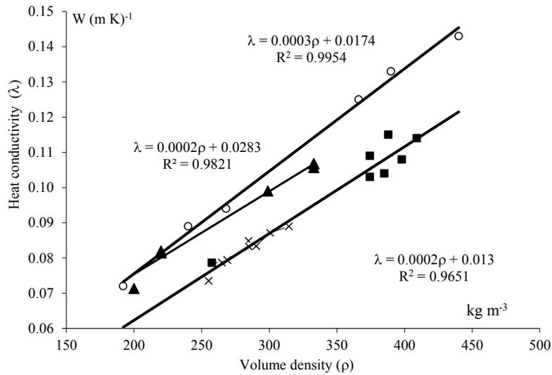
○ - Foam alfa gypsum (Skujans, Vulans et al., 2007), ■ - Foam β- Fogypsum, × - Foam β gypsum with hemp, ▲ - Alfa foam gypsum
