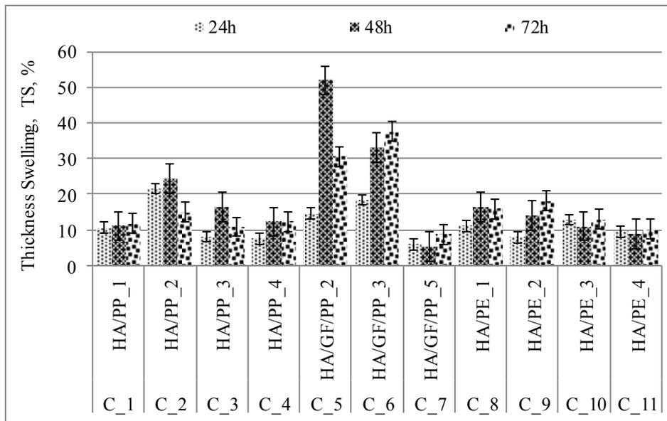
Figure 6. Composite thickness swelling TS, %
