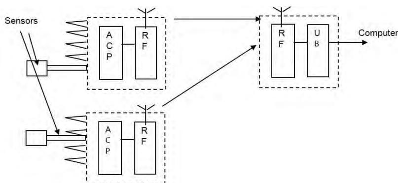
**Figure 1.** Block scheme of two-channel wireless heat flow and electronic measuring system MBox; ACP – analog-to-digital converter; RF – 2.4 GHz transmitter sending data to receiver module
