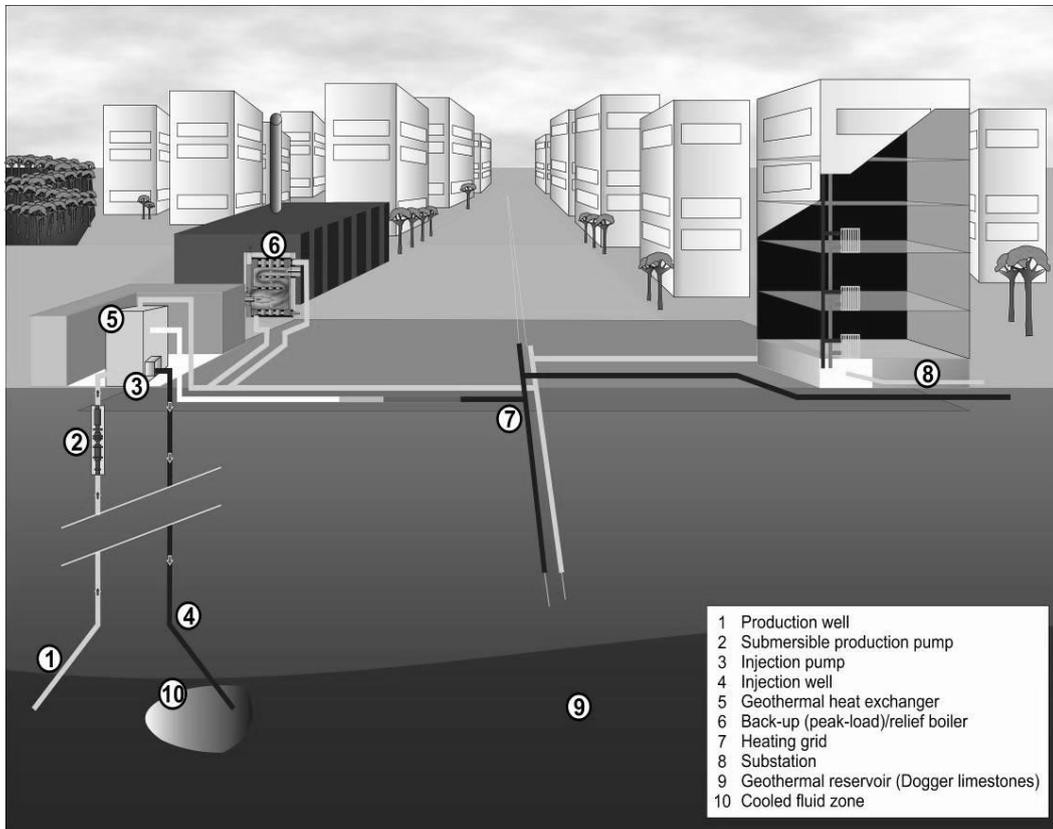
Figure 6. Geothermal doublet system for district heating (GeoDH, 2014)
