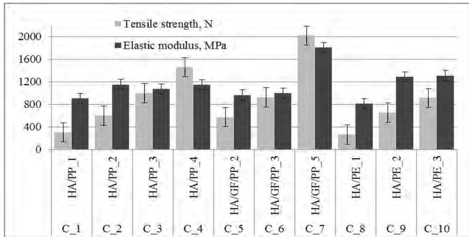
**Figure 3.** Composite Tensile Strength, N and Elastic Modulus, MPa
