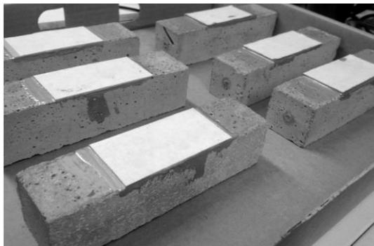
Figure 2. Samples with attached photoelastic plates
