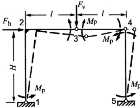
Figure 3. Combined mechanism
