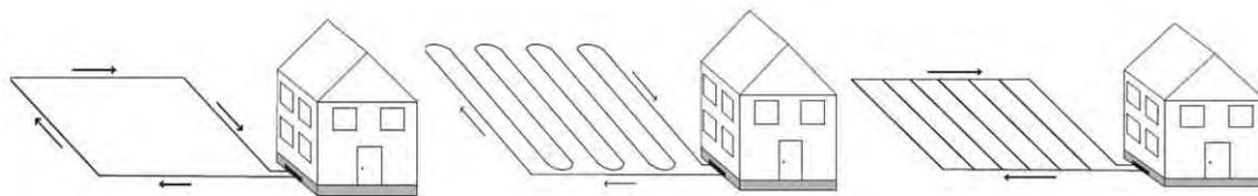
**Figure 4.** Horizontal loop heat exchange system configurations for geothermal heat pump from the left basic, in series, parallel (Self, 2013)
