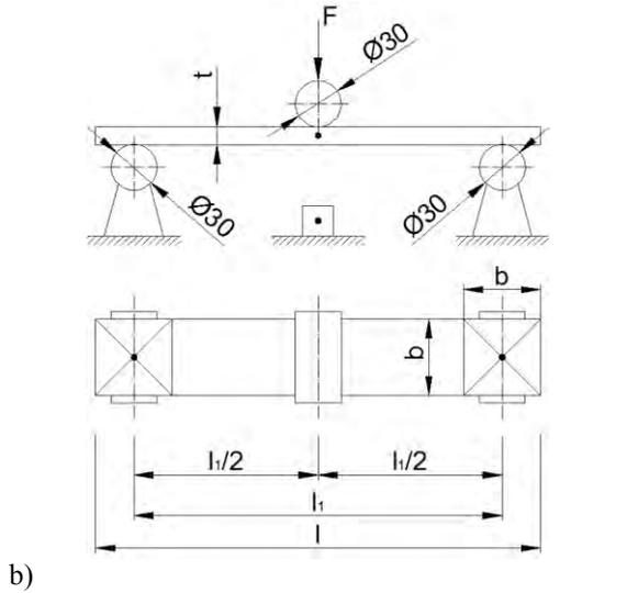
**Figure 1.** A photo of three-point bending test and of the Advanced Video Extensometer 2663-821 in the upper right corner (a); schematic view of three-point bending test; location of testing area for determining static hardness and thickness swelling (b)
