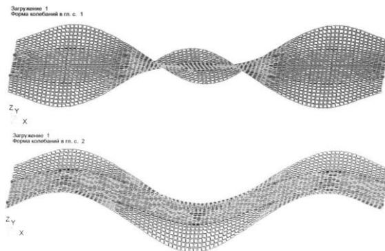
Figure 4. 1<sup>st</sup> and 2<sup>nd</sup> mode shape of bridge over Gauja in Valmiera
