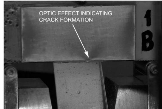
Figure 4. Sample B1 – phase I, moment of occurrence of photoelastic effect in the tensile zone of the beam
