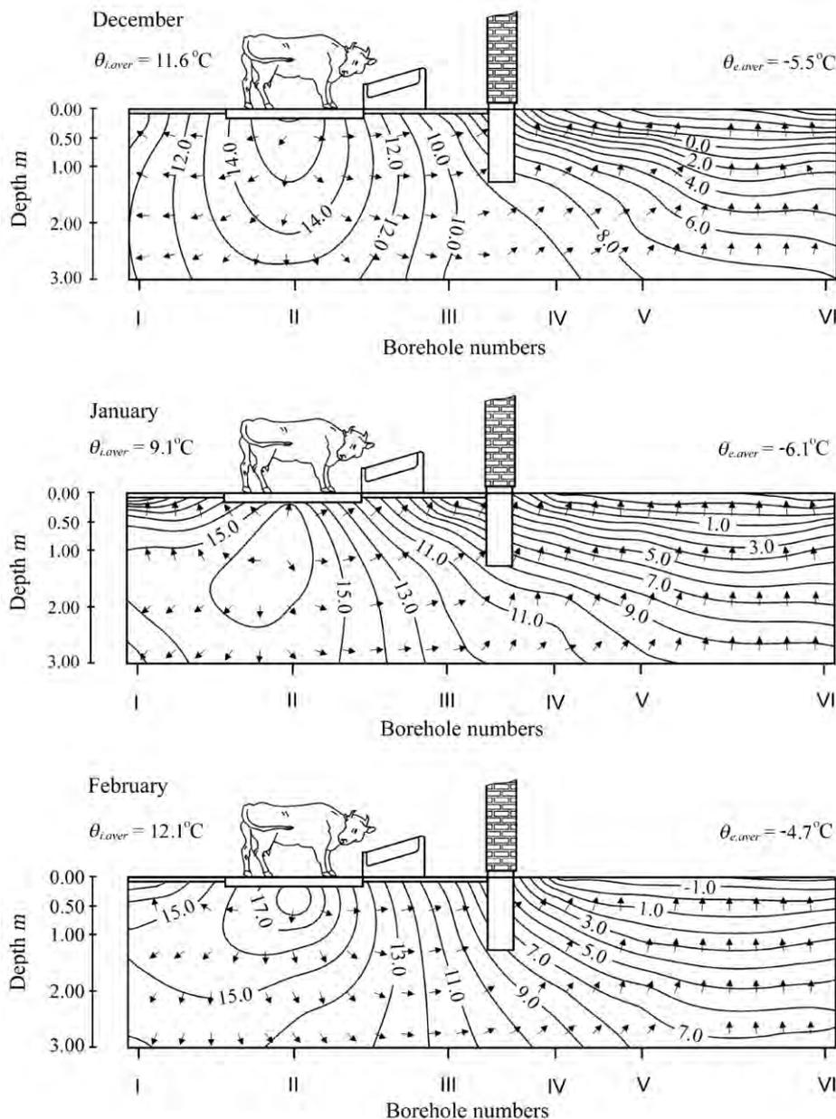
**Figure 2.** Distribution of the cowshed building base and environmental ground temperature during the period of the coldest indoor months
