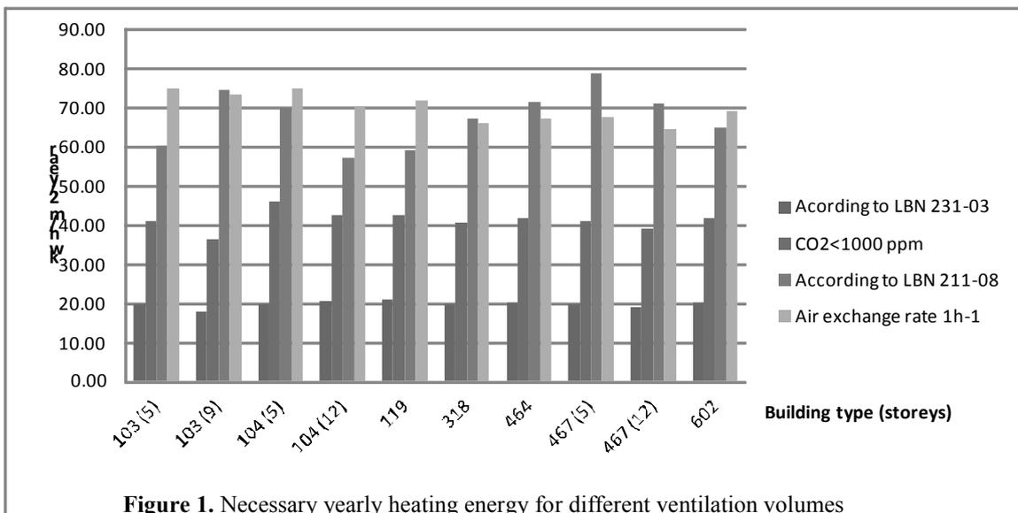
Figure 1. Necessary yearly heating energy for different ventilation volumes
