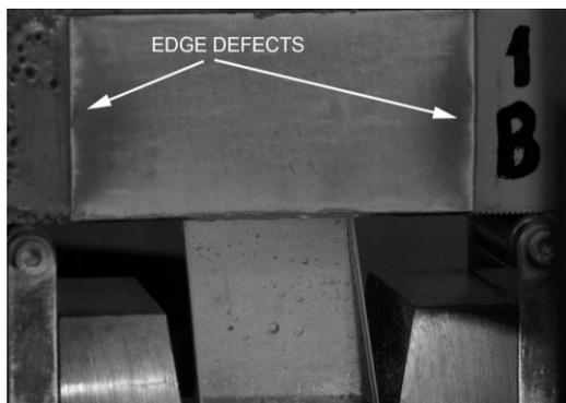
Figure 3. Sample B1 – element without applied load
