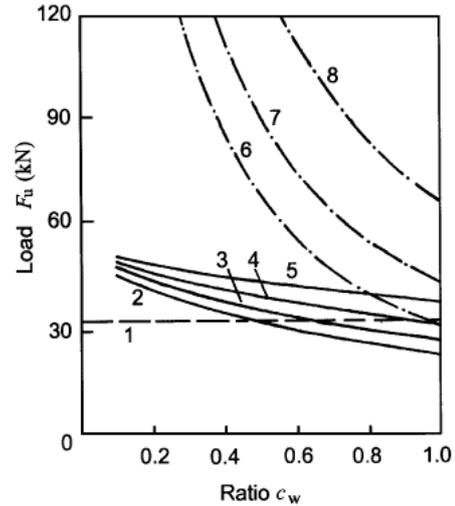
**Figure 4.** Ultimate load analysis at  $c_g = 1$ : 1 – beam-type mechanism; combined mechanism:  $k = 1(2)$ ,  $0.75(3)$ ,  $0.5(4)$ ,  $0.25(5)$ ; panel-type mechanism:  $k = 1(6)$ ,  $0.75(7)$ ,  $0.5(8)$
