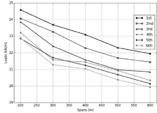
Figure 13. Calculated loads for highway's A1 Lane2
