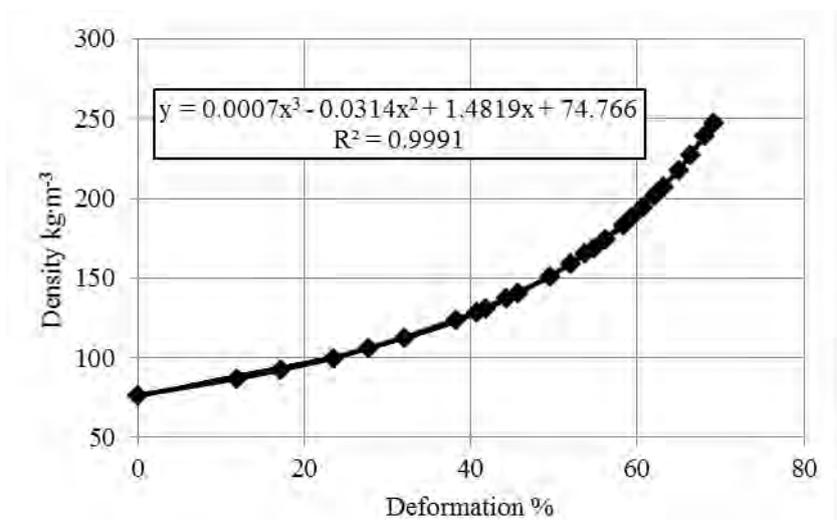
Figure 9. Dependency between compression deformation and density of triticale straw
