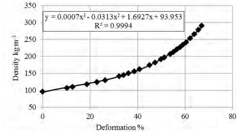
Figure 10. Dependency between compression deformation and density of rye straw
