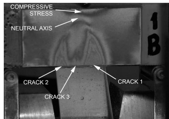
Figure 6. Beam B1 – phase II – beam with three cracks
