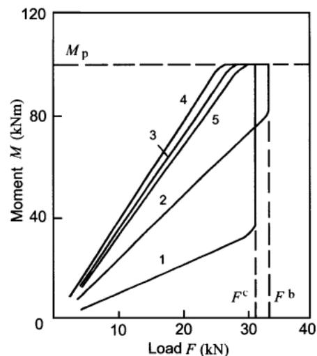
**Figure 5.** Mechanism type FEM analysis at  $k = 1$  and  $c_g = 1$ ;  $M_1^c$  (1),  $M_2^b = M_4^b$  (2),  $M_3^b = M_5^c$  (3),  $M_4^c$  (4),  $M_5^c$  (5)
