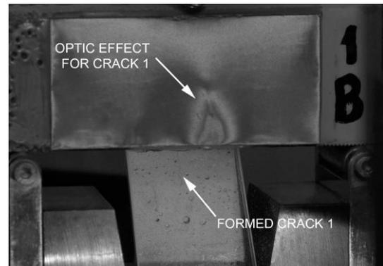
Figure 5. Beam B1 – phase II – cracked beam
