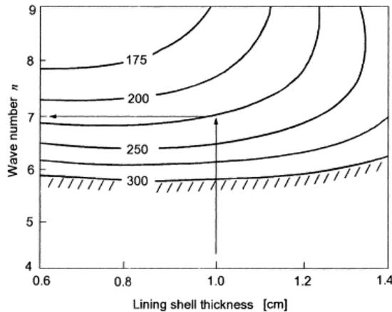
**Figure 3.** Isolines of critical temperature interval ( $^{\circ}\text{C}$ ) of lining shell:  $m = 1$ ,  $K_0$  0.75 MPa,  $L = 20$  m,  $R = 2.5$  m
