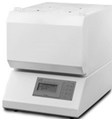
Figure 2 Straw sample for thermal conductivity test and „LaserComp“ FOX200 test apparatus
