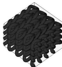
Figure 1. Structure of weft knitted fabric laminate (created in WeftKnit software (KU Leuven))
