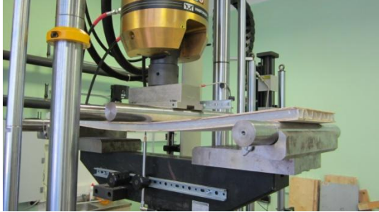
Figure 3. Bending set-up on INSTRON 8802
