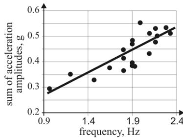
**Figure 10.** Relationship of amplitude and pacing frequency (longitudinal, ascend)
