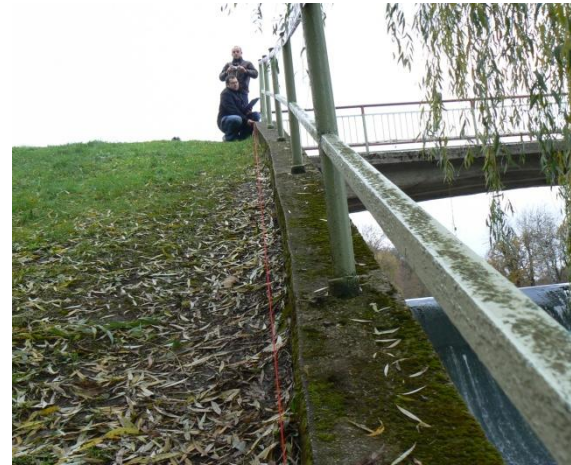
Figure. 2 Illustration of retaining walls deformations' measurements
