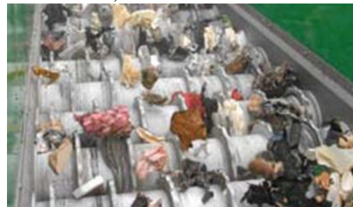
(b) The disc screen in Daibe (photo from: www.komptech.com)
