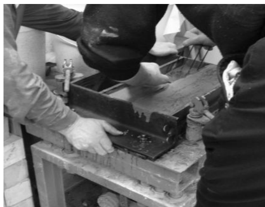
Figure 2. Combing fibers on the vibrating table
