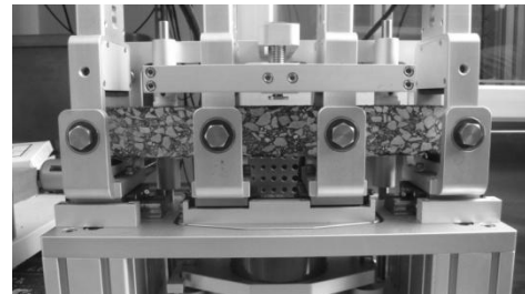
Figure 4. Test equipment for fatigue test
