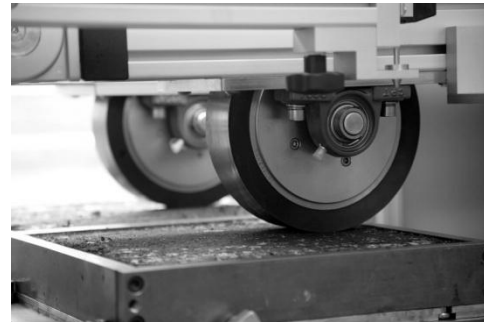
Figure 3. Test equipment for wheel tracking test
