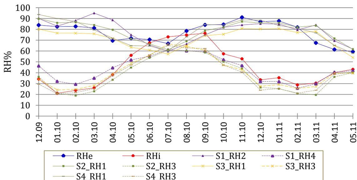
**Figure 8.** The relative humidity of various test walls [RH%], taking into account the average monthly value from December 2009 to May 2011 in the different layers of the walls
