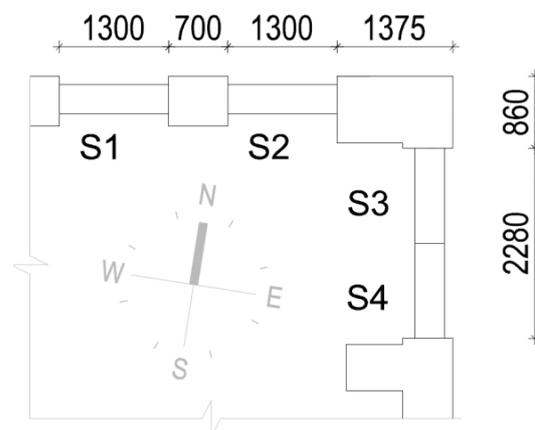
b) S1 – wall built of light clay blocks insulated with hemp chips
