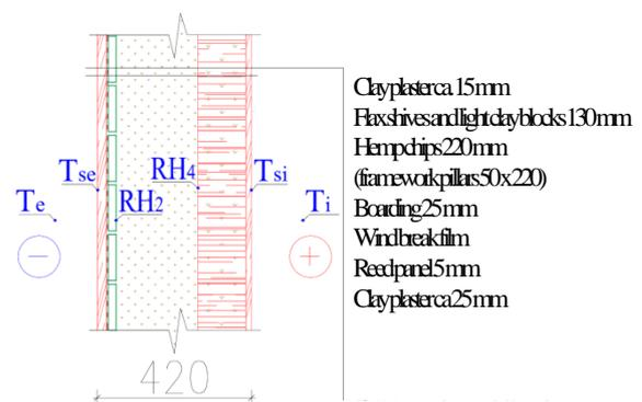
c) S2 – test wall built of horizontal reed
