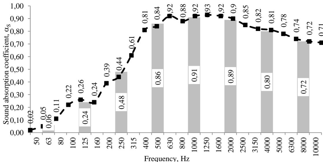
**Figure 6.** Measurement of sound absorption coefficient in a reverberation chamber. Frequency response curve of 1/3 octave bands foam gypsum with production technology w/g ratio 0.6, SAS 4 ml. — -  $\alpha$  value measured frequency response (1/3 octave band); ■ - Absorption coefficient,  $\alpha$ , average octave bands
