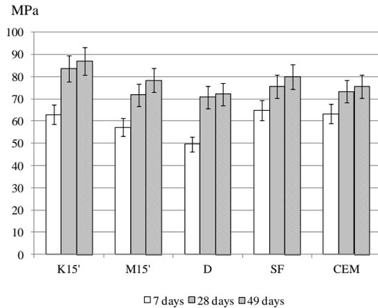
**Figure 4.** Compressive strength results: K15' - with metakaoline ground for 15 min., M15' - with calcined illite clay ground for 15 min, D - with dolomite powder, SF - with silica fume, CEM - cement without admixtures
