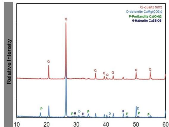
**Figure 6.** X-Ray diffraction results: mix D (below) with dolomite powder and mix SF (above) with silica fume
