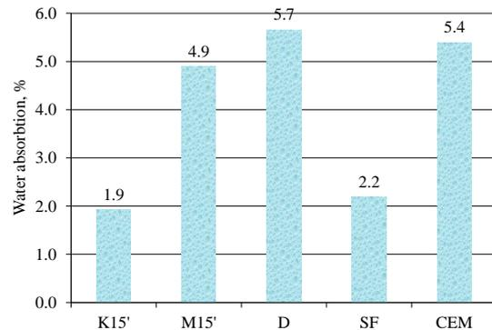
**Figure 5.** Water absorption results: : K15' - with metakaoline ground for 15 min., M15' - with calcined illite clay ground for 15 min, D - with dolomite powder, SF - with silica fume, CEM - cement without admixtures
