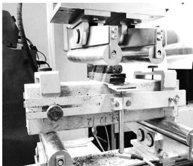
Figure 5. Testing device with fiber reinforced concrete prism
