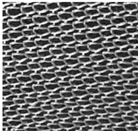
**Figure 3.** Knitted fabric for concrete shell reinforcement
