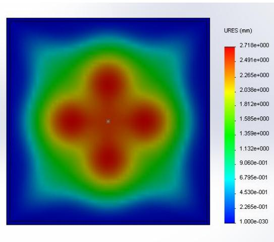
**Figure 10.** Vertical displacement in loaded shell.
