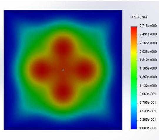
**Figure 10.** Vertical displacement in loaded shell.
