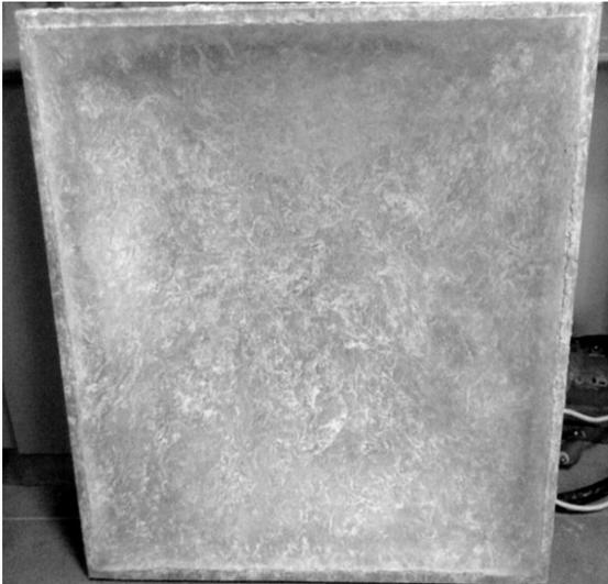
**Figure 4.** Short glass fiber concrete shell
