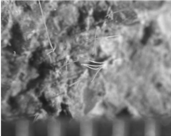
**Figure 18.** Micro synthetic fibers on a macro-crack surface
