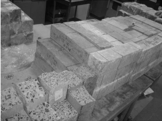
**Figure 10.** Samples tested for four point bending
