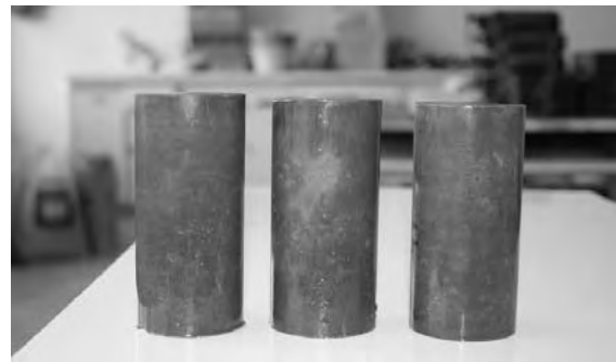
Figure 3. The specimens prepared by 10 MPa pressure application.
