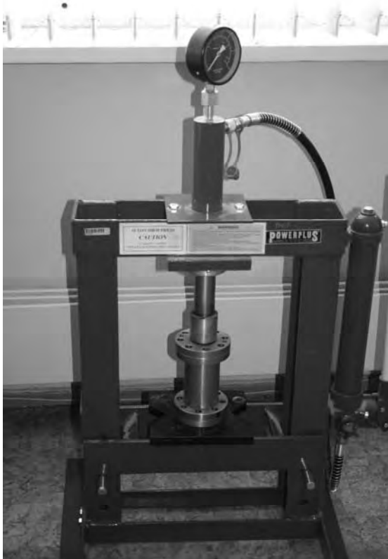
Figure 2. Experimental setup for pressure application to the specimens.
