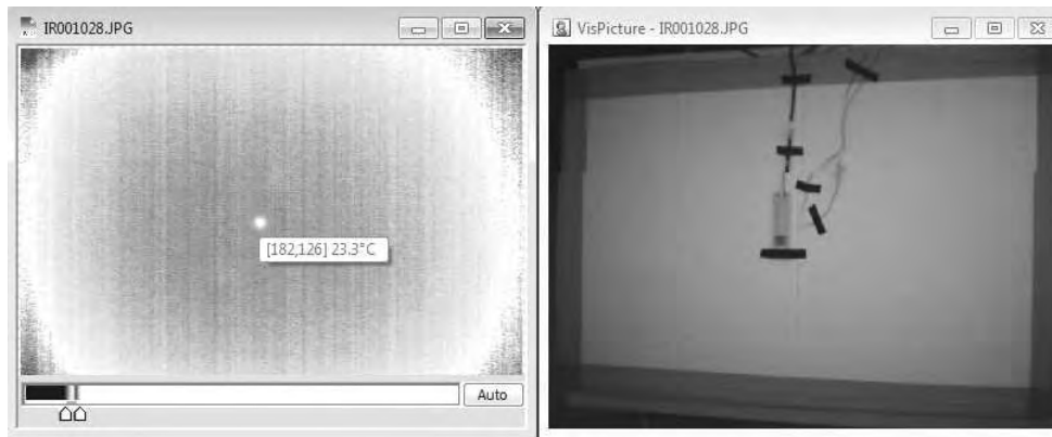
Figure 6. Measurements of the surface temperature with ThermoPro TP8 ( \epsilon=0.90 ). Analysis made in the programme Guide IrAnalyser.
