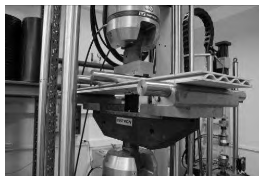
Figure 5. Sandwich panel in 4-point bending test set-up on INSTRON 8802.
