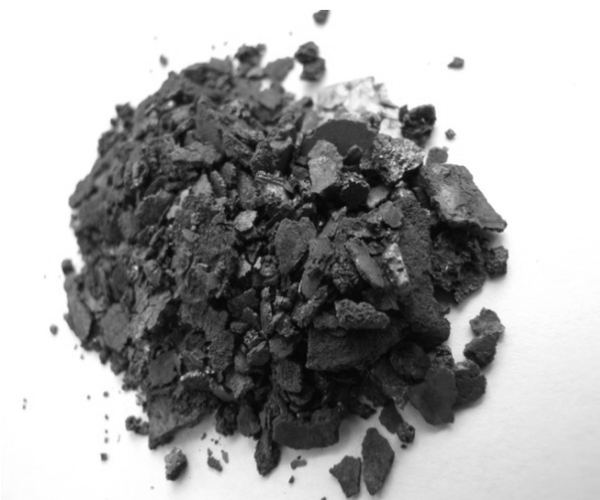
Figure 4. Raw mill scale from JSC “Liepajas Metalurgs”.
