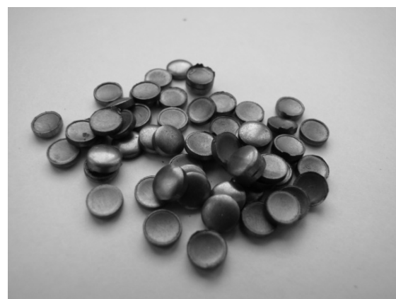
Figure 6. Steel punching from JSC “DITTON Driving Chain Factory” (Latvia). Diameter 3.0 \div 10.8 \text{ mm} , height 0.5 \div 3.3 \text{ mm} . The specific gravity of steel punching is 7800 \text{ kg/m}^3 .
