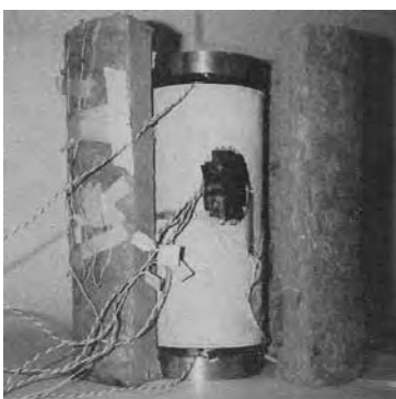
Figure 10. Concrete cylinder with insulating layers and wood fiber plates at cylinder ends with thermocouples.
