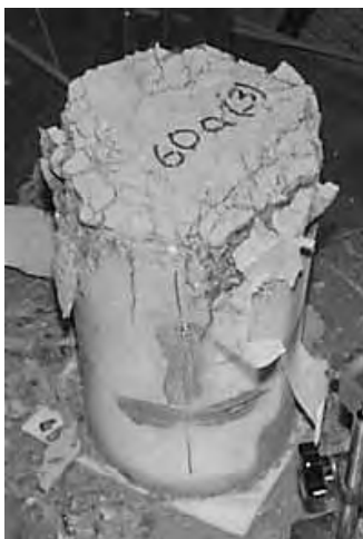
Figure 8. With two Teflon layers to reduce friction, the concrete cylinder completely disintegrates at compressive failure. Vertical cracks show up.
