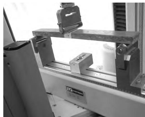
**Figure 1.** Three-point bending and points of deflection measurement: a) scheme b) photo
