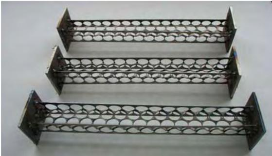
Fig.9. Perforated struts before pressure strength test
