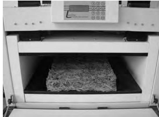
**Figure 6.** Thermal conductivity test.
