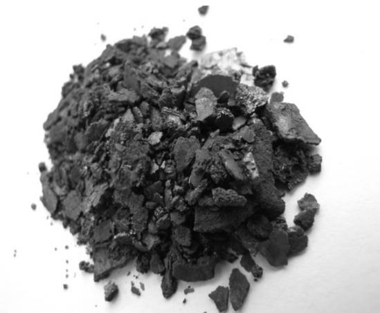
**Figure 4.** Raw mill scale from JSC “Liepajas Metalurgs”.
