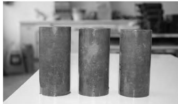
**Figure 3.** The specimens prepared by 10 MPa pressure application.
