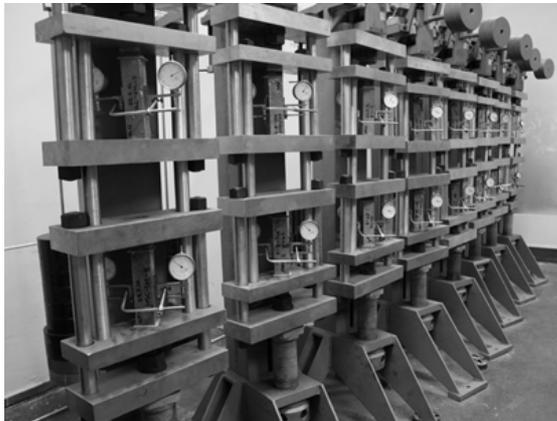
**Figure 3.** Specimens in the creep lever test stand
