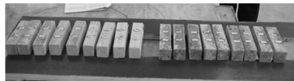
Figure 2. Specimens with aluminium plates.
