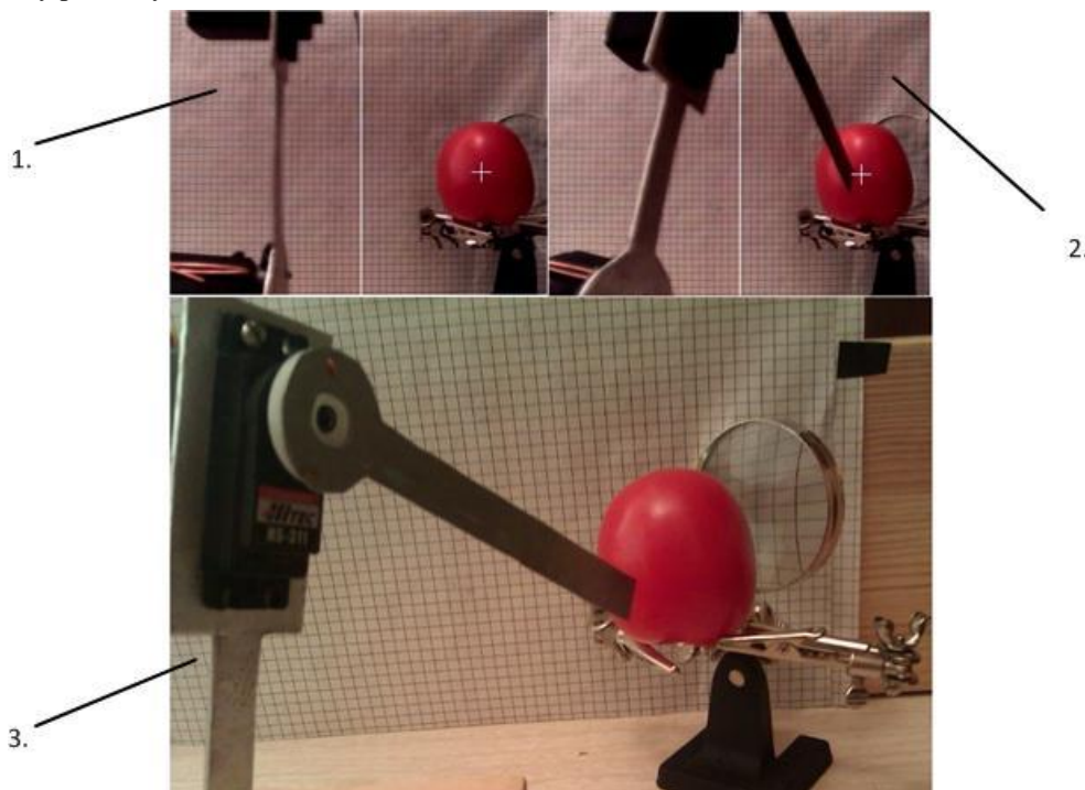
Fig. 10. Tomato detection: 1. – tomato recognition (web camera view), 2. – manipulator pointing to tomato (web camera view), 3. – whole situation from side view.
