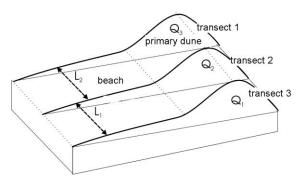
Fig. 5. Parameters used for primary dune deposits volume calculation [created by author]
