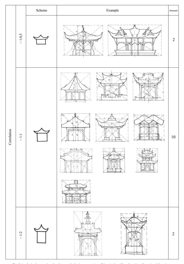
Fig. 3. Analysis of proportional and metro-rhythmic construction of historical pavilions based on dimensional drawings.
