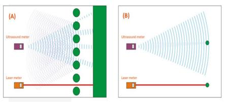
**Figure 3.** Limitations on the use of ultrasonic rangefinders (source: www.transcat.com)
