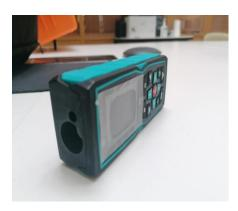
Figure 4. Laser rangefinder Stonex M6 used in the study (source: author's photo fixation)
