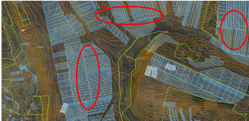
Fig. 4. Fragment of location of land shares by longer side along the slope (Poliana village council, Lviv region)
