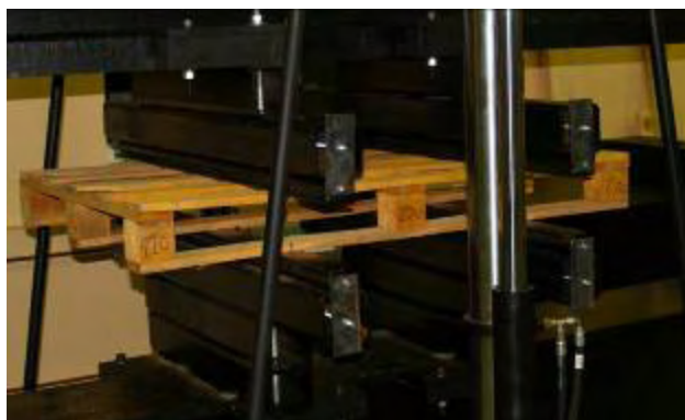
5. att. Koksnes paliktņu pārbaudes. Fig. 5. Testing of wooden pallets.
