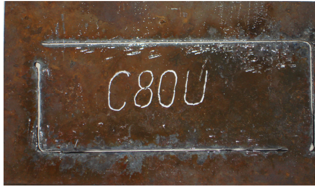
Fig. 1. The shape and cutting trajectory of steel sample C80U
