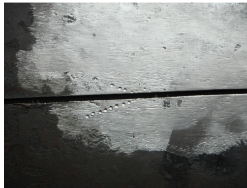
Fig. 2. Sample of hardness measuring HRC in cutting area
