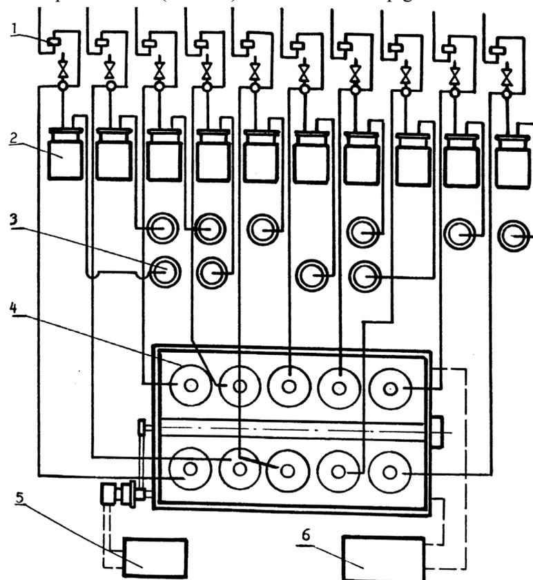
Fig. 1. Unit for anaerobic fermentation of biomass: 1 – pressure gauge, 2 – gas cylinder, 3 – receptacle for liquid, 4 – container with bio-reactors, 5 – automatic mixing unit, 6 – automatic temperature maintenance unit
