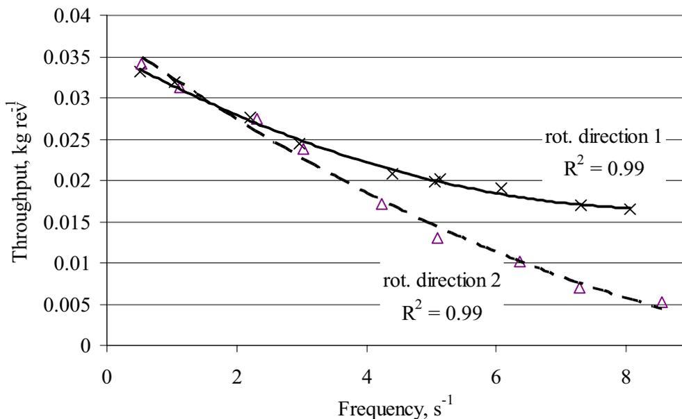
Fig. 3. Throughput of the spools feeder vs. rotation frequency
