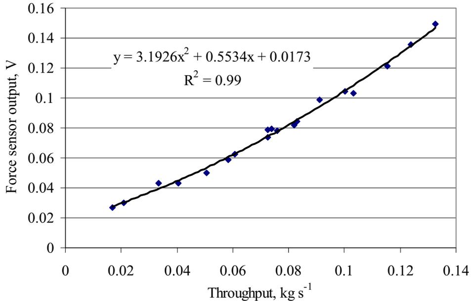
Fig. 4. Force sensor output voltage vs. mass throughput
