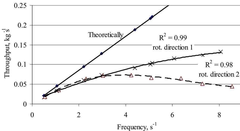
Fig. 2. Throughput of rotary spools feeder in dependence on frequency
