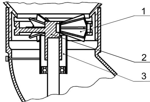
Fig. 1. The feeder with radial located spools:
