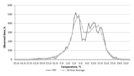
Figure 5. Hourly temperature distribution for TRY and 30-year average data.
