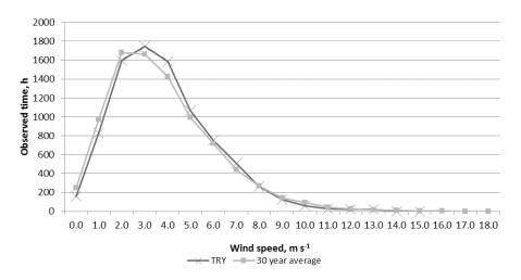
Figure 6. Wind speed distribution for TRY and 30-year average data.
