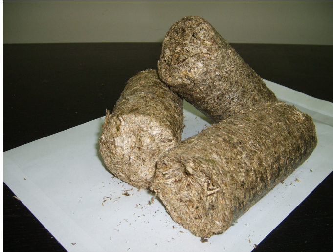
Photo 2. Briquettes made of hemp shives
