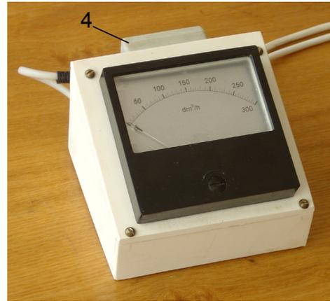
Figure 2. Frequency-voltage convertor
