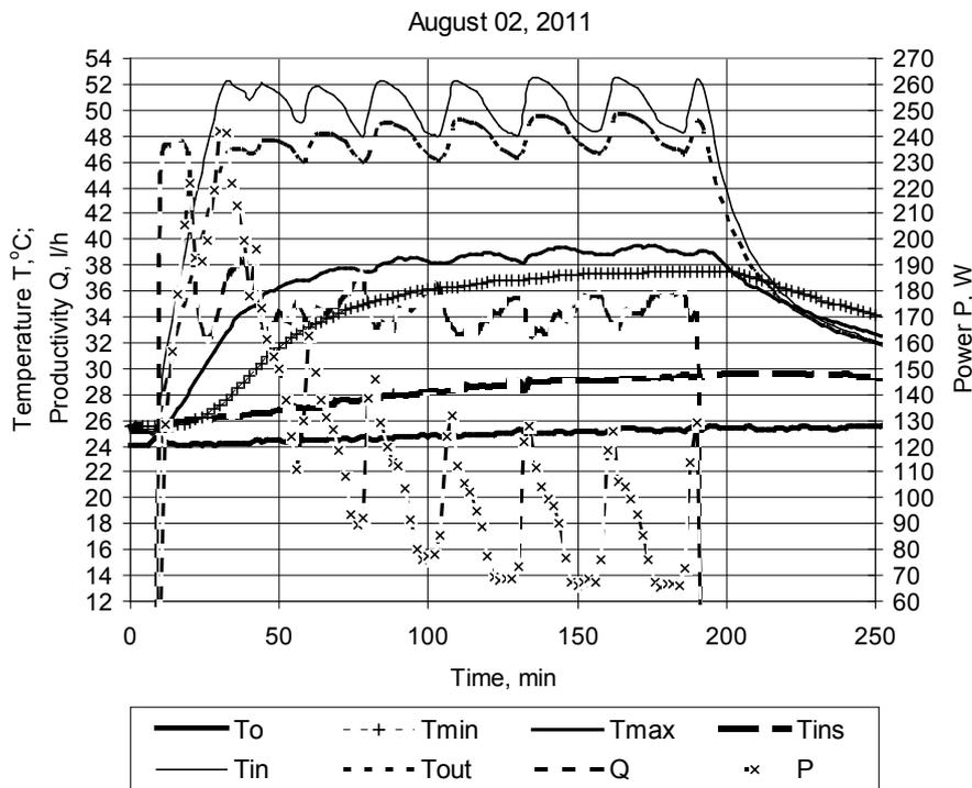
Figure 9. Experimental results of the temperature distribution in the heated floor panel using the invented device:  $T_o$  – surrounding air temperature,  $T_{min}$  and  $T_{max}$  – the lowest and the highest temperature on the panel's surface,  $T_{ins}$  – temperature inside the panel,  $T_{in}$  and  $T_{out}$  – inflow and outflow heat carrier temperature,  $Q$  – efficiency of the heat carrier circulation pump,  $P$  – heat power consumed by the panel.
