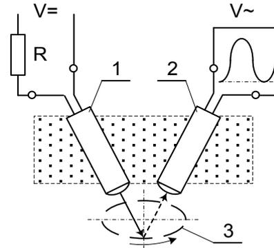
Figure 4. Infrared irradiative diodes: 1 – VD1; 2 – VD2
