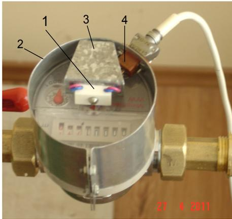
Figure 1. Heat carrier flow intensity metering sensor
