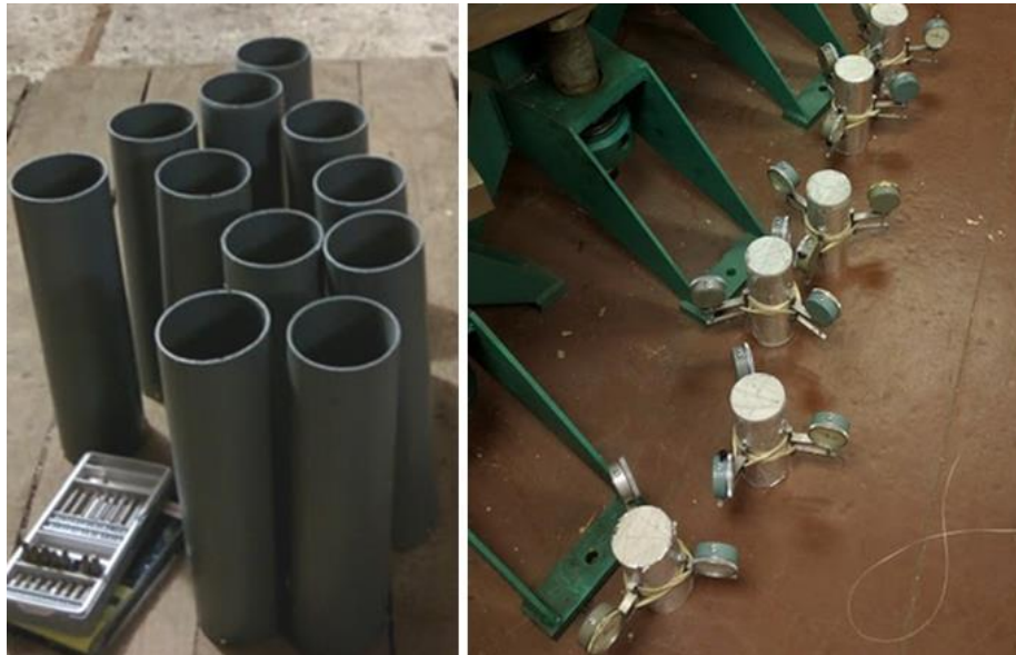
Fig. 2 Cylindrical moulds (at the left) and specimens with tensometers attached (at the right)
