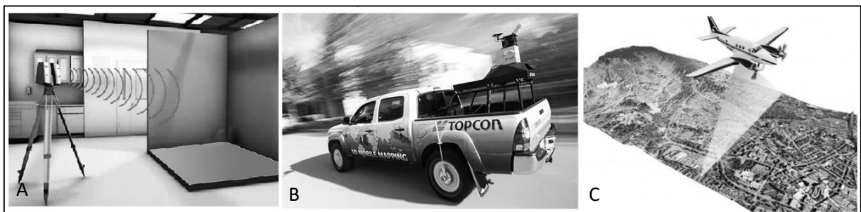
Fig. 1. Methods of laser scanning: A) static laser scanning in room on a tripod [16]; B) mobile laser scanning outside from the car [17]; C) aerial laser scanning from an aircraft [15]
