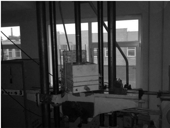
**Figure 1.** Straw pressure test with universal testing machine
