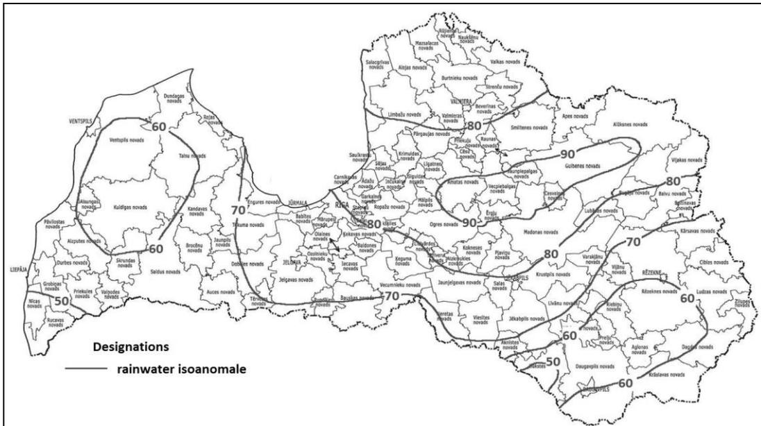
**Figure 1.** Maximum stormwater runoff module  $q_{20}$  with the probability of 100%;  $l(s*ha)^{-1}$
