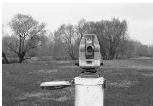
Figure 6. Total station on the baseline in Hlohovec
