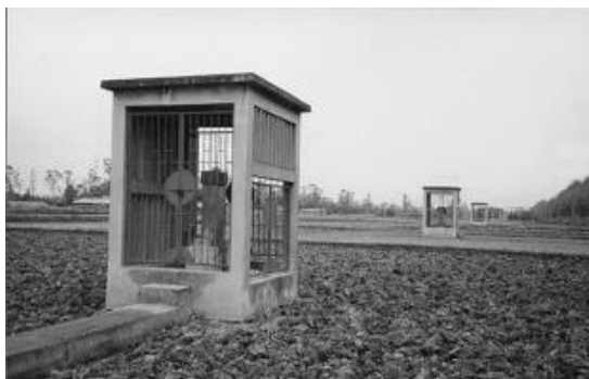
Figure 4. The look of calibration base pylon in China
