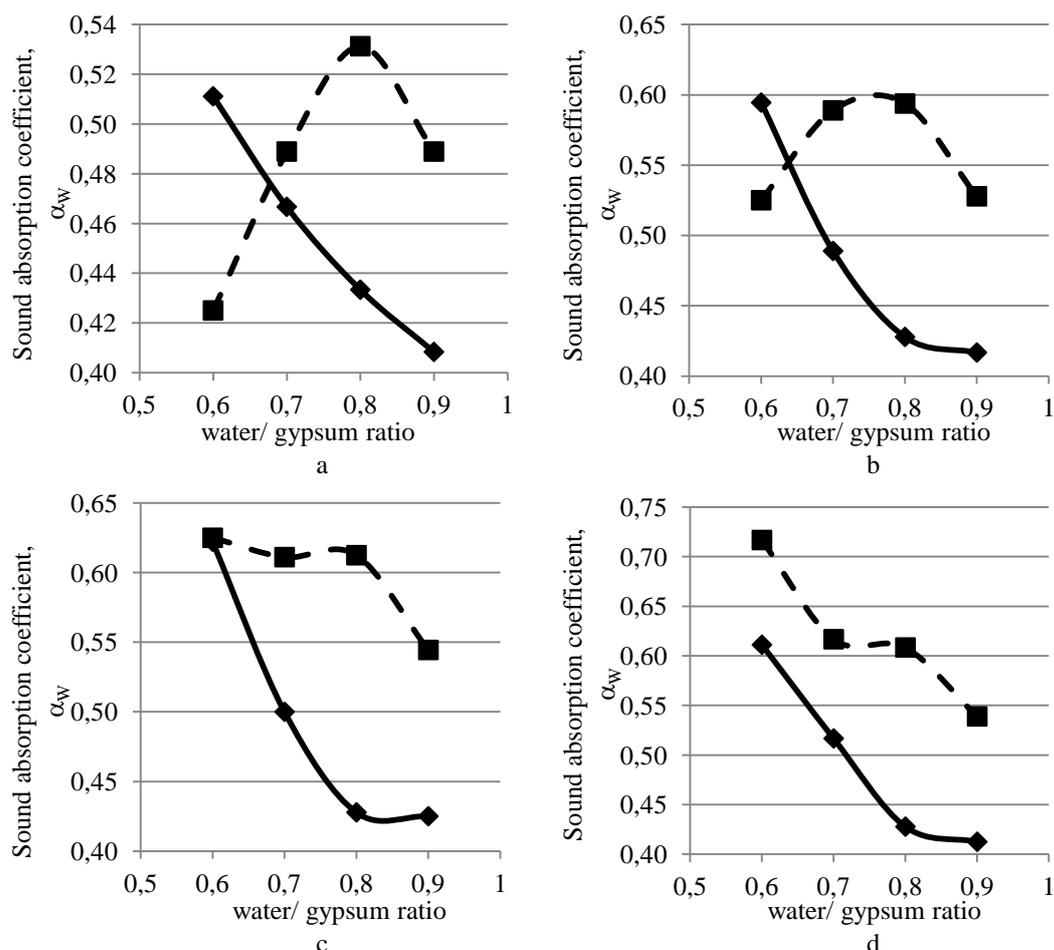
**Figure 5.** Foam gypsum weighed average sound absorption coefficient at different production technology. — SAS 4 ml; - - SAS 6 ml, a-30 mm thick sample; b-40 mm thick sample; c-50 mm thick sample; d-100 mm thick sample
