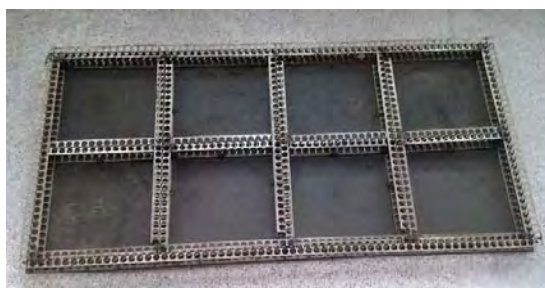
Fig.14. Shield block made using reinforced-rubber and perforated profiles.
