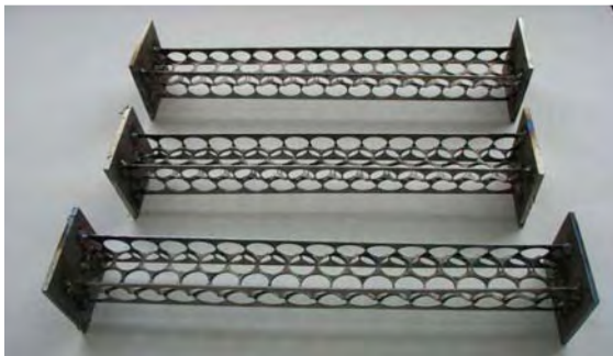
Fig.9. Perforated struts before pressure strength test
