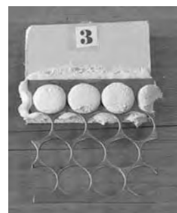
Fig.8. Connection of perforated steel band and gypsum plate with adhesive on gypsum basis.
