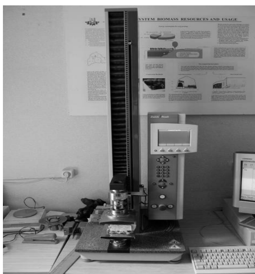
Figure 2. Company „Zwick” device for testing bending and pressure resistance.
