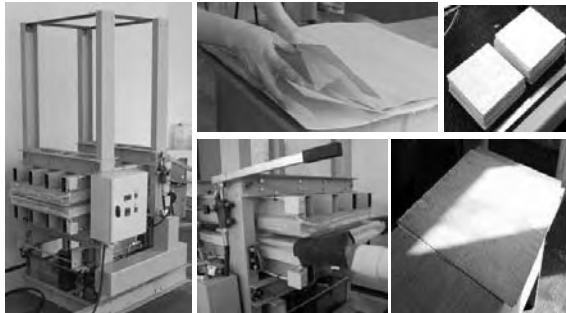
Figure 2. Experimental production of laminated composites.
